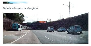
It appeared that the difference in contrast between these road surfaces interfered with lane keeping systems, either leading vehicles out of their lane, or disengaging lane keeping.
