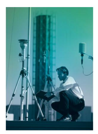
Monitoring air quality adjacent to the Domain Tunnel vent stack.
